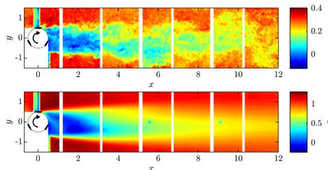
Figure 1: Instantaneous (top) and mean (bottom) streamwise velocity for the VAWT
